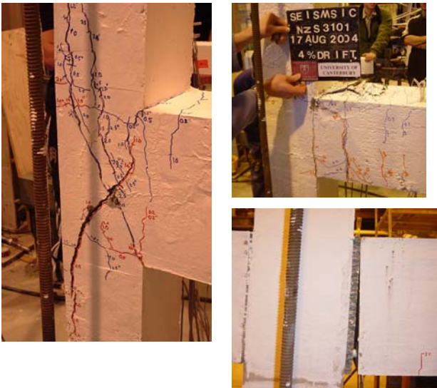
Figure 15. Evolution of seismic resisting connections: performance of beam-column joints designed according to pre-1970 codes (shear damage in the joint); following capacity design principles as per the NZS3101:1995 (beam plastic hinge) and adopting hybrid jointed ductile connections as per NZS3101:2006 (controlled rocking system).
