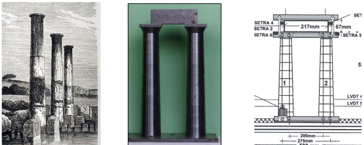
Figure 28. Left: Representation of the ruins of a Greek temple after an earthquake event. Reduced stability due to the loss of axial load contribution from the above temple. Centre and right: Experimental shake table test on multi-block ancient-type column specimens adopting vertical SMA wires (Manos et al., 2000) in order to improve the structural stability and capacity to sustain future earthquake eventson a square column.
