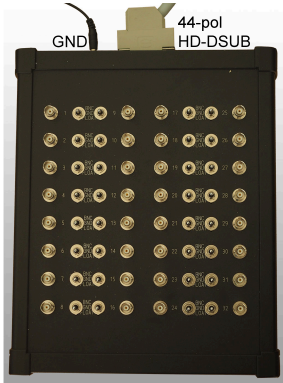
Figure 2.11: The 32pin BNC breakout box used to connect the measuring inserts (via a 44 pin High Density D-Sub connector, see top of figure) with the devices. The grounding wire can be seen on the left side.
