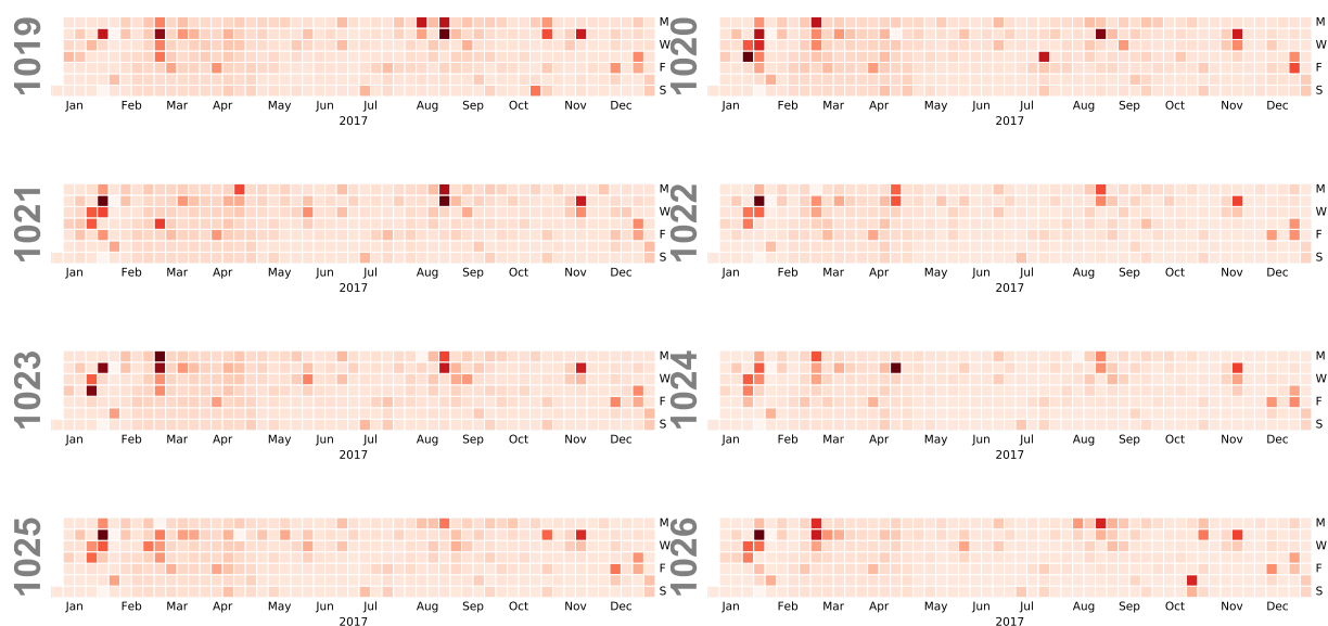
Figure 5.7: Similar patterns of syslog generation by various nodes within the rack 2 of Island 1 in Taurus. Each cell shows the number of entries generated per day during the year 2017. Darker colors indicate higher number of syslog entries.
