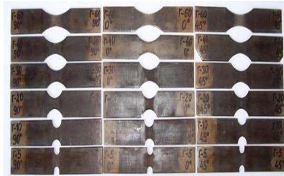
Fig.2 - Photograph of test tubes stretched to the maximum force
