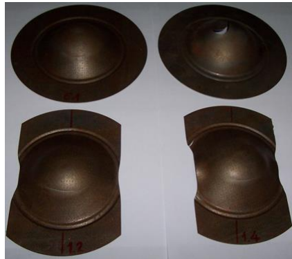
Fig.4 - Drawn parts of circular plates and sheet strips to limit deformability
