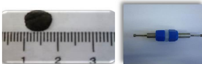
Figure 3.7 Swagelok type cell assembly and electrode representation
