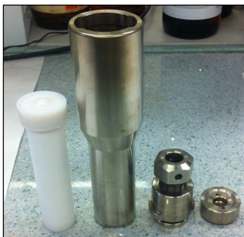
Fig. 5.2.2 Steel autoclave and teflon liner used for hydrothermal synthesis.
