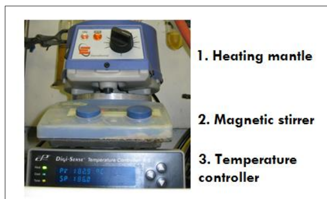
Fig. 4.2.2 Heating mantle, magnetic stirrer and Proportional-Integral-Derivative (PID) temperature controller used during the synthesis of Zn_xCo_{1-x}Fe_2O_4 nanoparticles.
