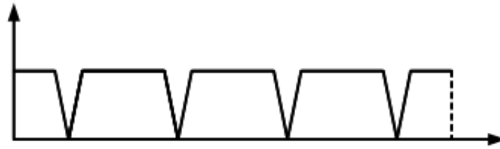
Figure 3.1: Non-Overlapping filterbank response.
