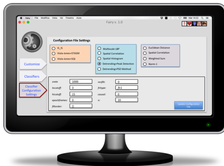
FIGURE 2.19: The form by means of which is possible to modify the configuration file.
