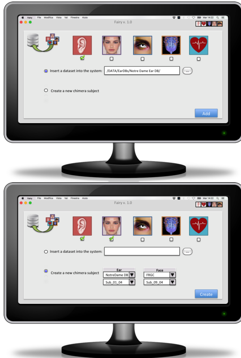
FIGURE 2.15: In the uppermost image the user adds the Notre Dame dataset to the FAIRY warehouse; in the bottommost, instead, a new chimera is generated.
