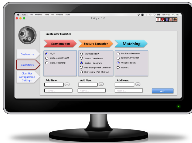
FIGURE 2.17: The user can add a new classifier to the platform or can compose a new classifier by cascading a segmentation method, a feature extraction method and a matching method.
