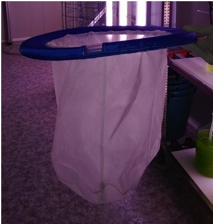
Figure 20 - Mesh basket used for tank cleaning.
