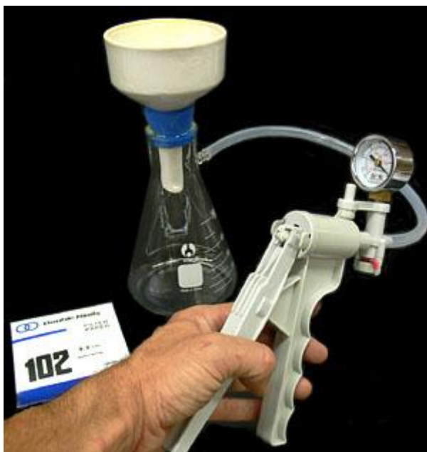
Figure 4.5: Manual vacuum pump connected to a filter flask.
