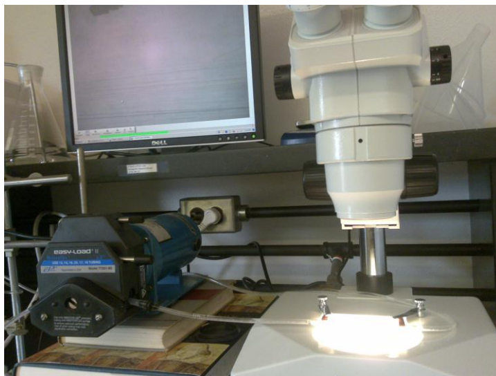
Figure 4.6: Online sampling device with the optical microscope and the peristaltic pump.
