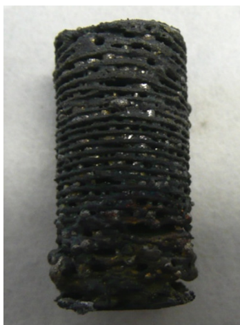
FIGURE 3-5: Image of the final sample obtained after the SHS reaction of one of the mixtures (system S2_R L 30) containing lunar regolith simulant.
