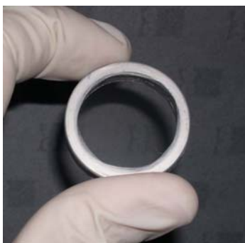
Figure 4.8: A Mylar® foil glued onto a circular frame.
