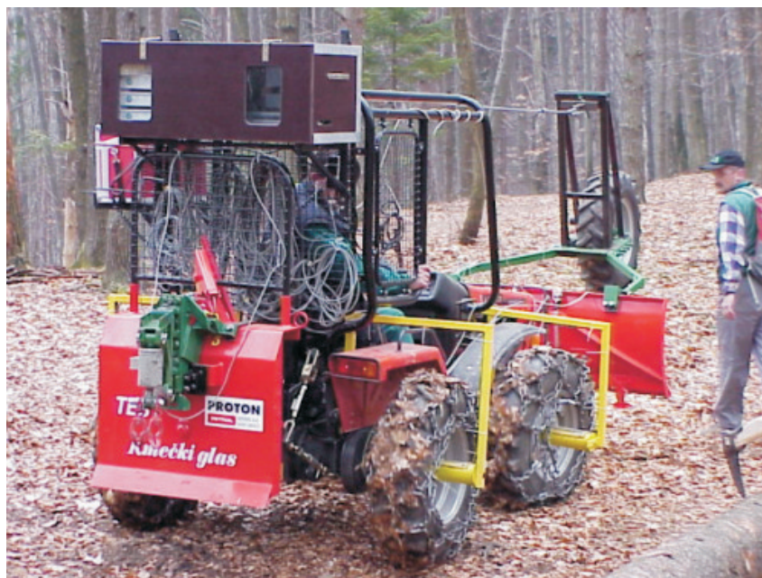
Fig. 1: AGT 835 with basic forestry equipment and measuring instruments during the test
