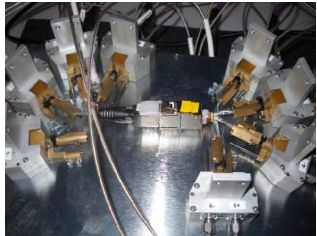
Figure 4-6: Cable clamp termination unit with test object
