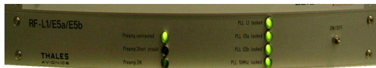
Figure 62: Front view of the RFU rack.
