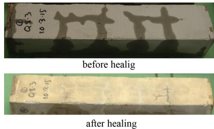
Figure 16. Typical water absorption performance before and after healing (at 2 hr water absorption).
