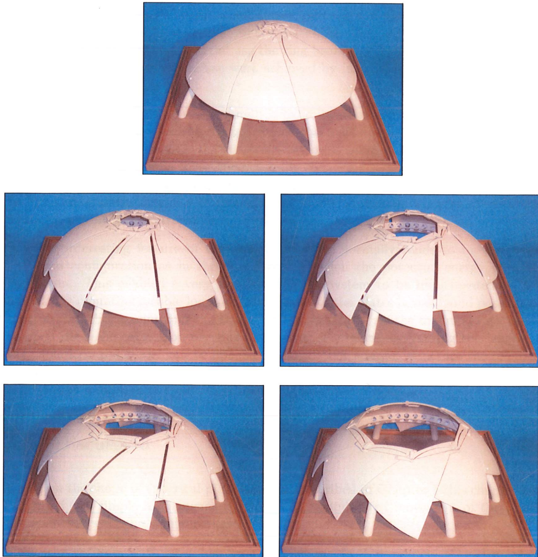
Figure 6.16: 400 mm span model fabricated using 3D Ink-Jet printing
