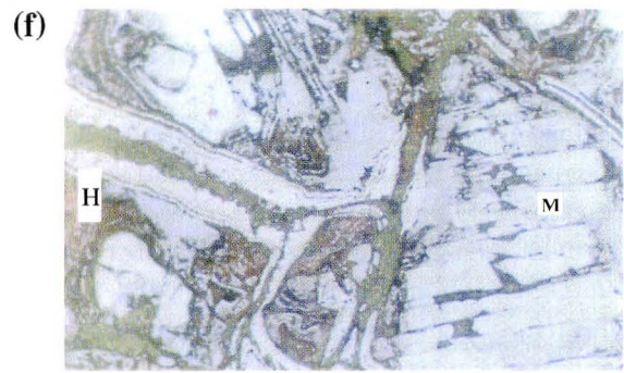
Photomicrograph showing Magnetite (M) and secondary aggregates of Hematite (H) 200X.
