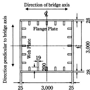
Fig. 2 Cross section ① (unit: mm)
