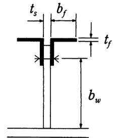
**Fig. 9** Details of retrofitting of existing longitudinal stiffener
