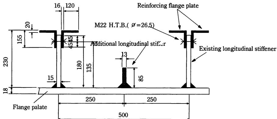
Fig. 11 Details of part B in flange plate (unit: mm)
