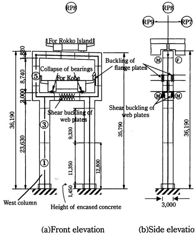
Fig. 1 Bridge pier under consideration and damage due to the Hyogo-ken Nanbu Earthquake (unit:mm)
