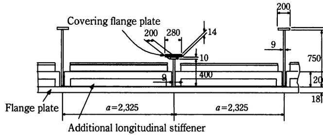
**Fig. 12** Reinforcement to transverse stiffener of flange plate (unit: mm)
