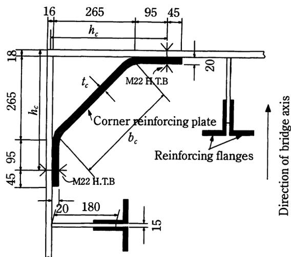
Fig. 5 Corner reinforcement (unit: mm)
