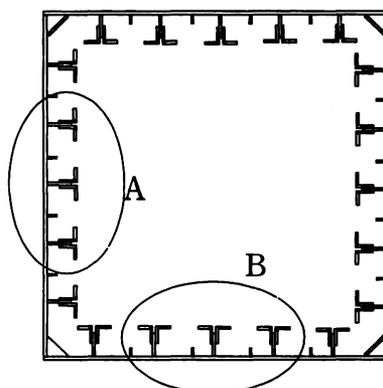
Fig. 6 Cross section of retrofitted bridge pier
