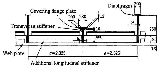
Fig. 10 Reinforcement to transverse stiffener of web plate (unit: mm)
