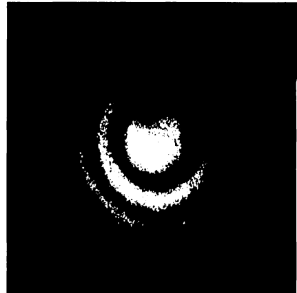
Fig. 7 Compensated interference fringe by modified Twyman-Green interferometer with SZP
