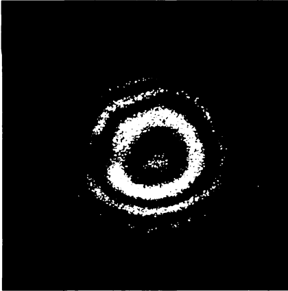
Fig. 6 Interference pattern by Twyman-Green interferometer with SZP
