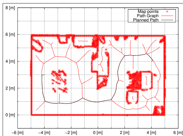
Figure 4.11: Planned path from (4\text{ m } 4\text{ m})^T to (-4\text{ m } 3\text{ m})^T containing 195 line segments forming the (optimal) path in the path graph. Four non-redundant paths can be found by A^* whereas the depicted one is the shortest regarding its total cost if form of travelled distance. The search took approximately 4.4 ms.
