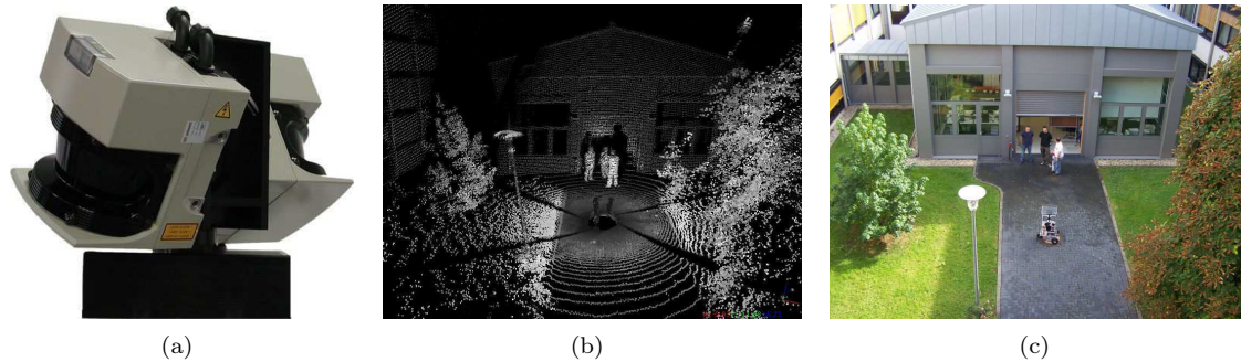
Figure 2.7: Continuously rotating 3D laser scanner (a) and example data (b) taken in front of the Robotics Pavilion at Fraunhofer IAIS. A photo of the scene is shown in (c). The color of the 3D points corresponds to the received remission values.
