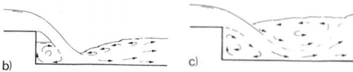
Figure 14. Flow pattern downstream of a sudden drop in a rectangular channel (Vischer & Hager, 1995).
