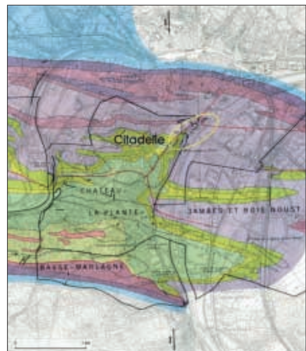
Figure 2a. Coal measures map of Basse-Sambre coal field with concession boundaries, location of Citadelle outcrops (encircled) and cross-section (line I-I) on fig. 3. Hatched line delimitates mined-out zones (adapted from Bouckaert, 1967).
