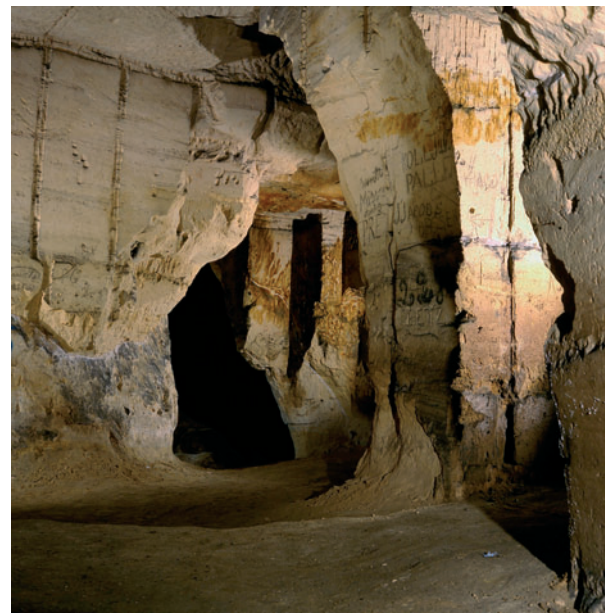
Figure 3: Underground quarry in Nekum calcarenitic limestone, extracted for 'maastrichtsteen' building stone, resulting in rectangular sections. Grote Kuil, Vechmaal (photo B. Odeur).
