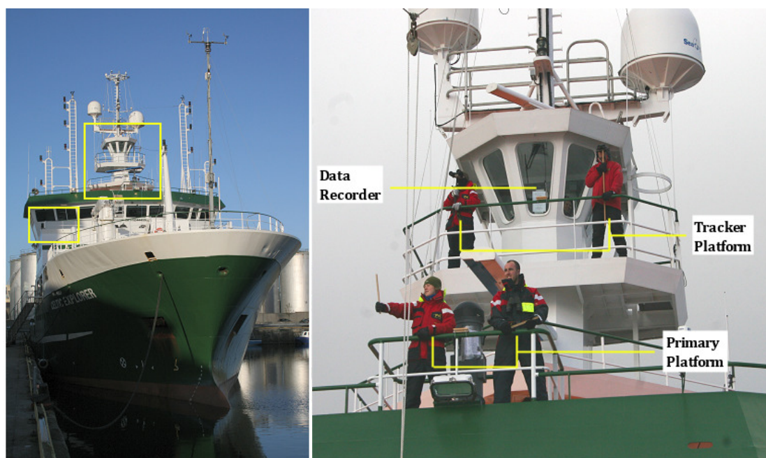
Fig. 2 Position of Cetacean survey and bird survey platforms on R.V. Celtic Explorer.
