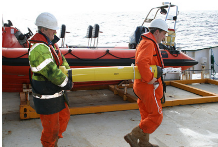
Fig. 34 ARGO float being brought on deck for deployment over the Porcupine Seabight.
