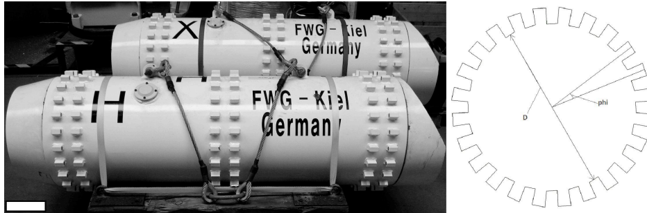
Figure 6.2 (left) Pre-deployment photo of the test mines. The white bar in the lower left corner represents 20 cm. (right) BRM cross-section with D (47 cm), diameter, and \phi , the angle between two successive LED housings. Mine burial diameter refers to the height of the mine (or mine ring) buried with respect to the lowest LED pair
