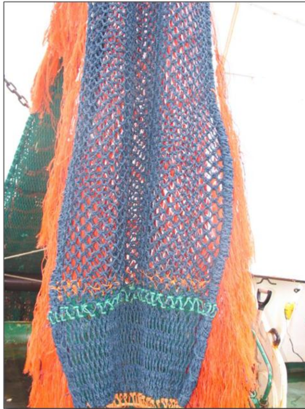
Fig. 15-1 – T90 and diamond meshes (top) and a T90 cod-end with a posterior sheet of netting (5 rows) with T0 orientation.
