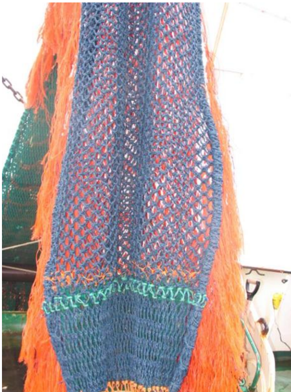
Figure 3-1 – T90 cod-end with a posterior sheet of netting (5 rows) with T0 orientation
