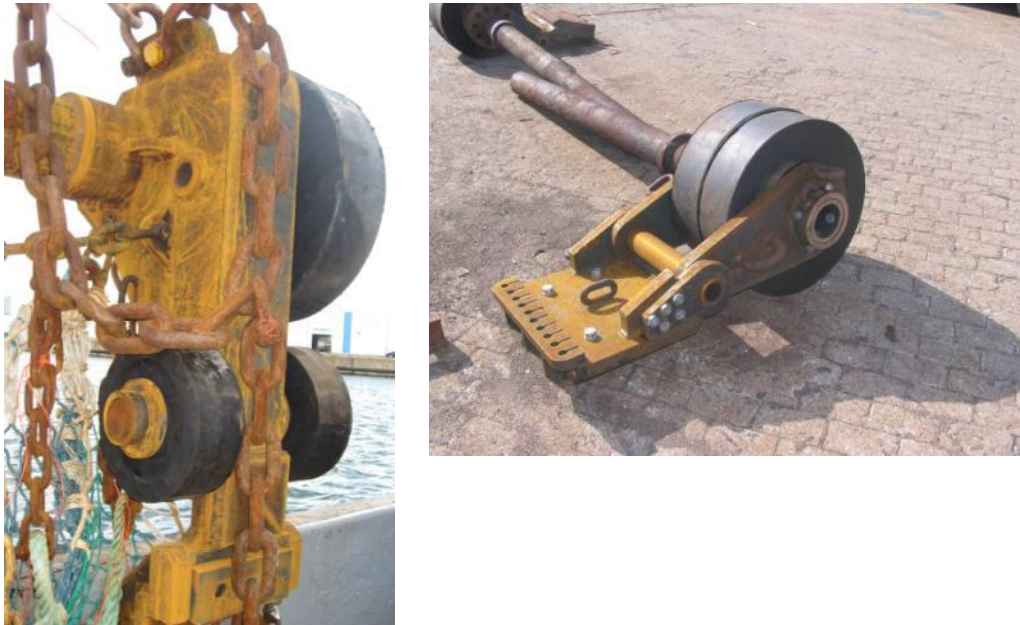
Figure 9-1 – wheeled trawl shoes tested in chain matrix beam trawl (left) and tickler chain beam trawl (right)
