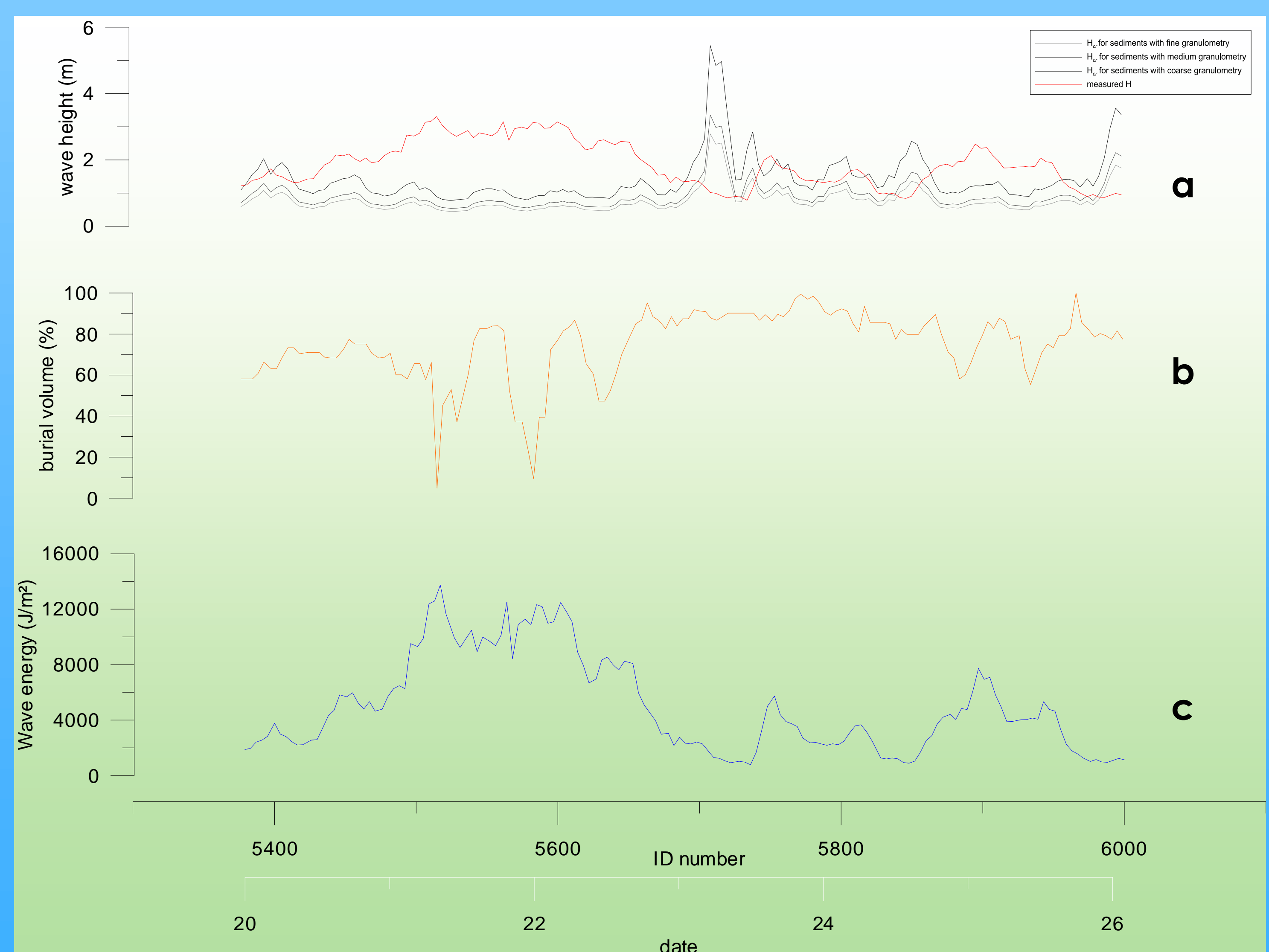
Fig. 6: storm in November 2008. (a): comparison between measured curve of real wave height (red) and calculated curves of critical wave height (different tone of grey); (b): curve of burial volume; (c): curve of wave energy.
