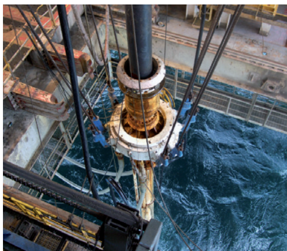
Figure 6.2. Riser and slip joint of a semisubmersible oil rig which carries oil and gas to the surface while drilling
