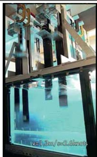
Test set-up of 4 wave cylinders in a wave flume
