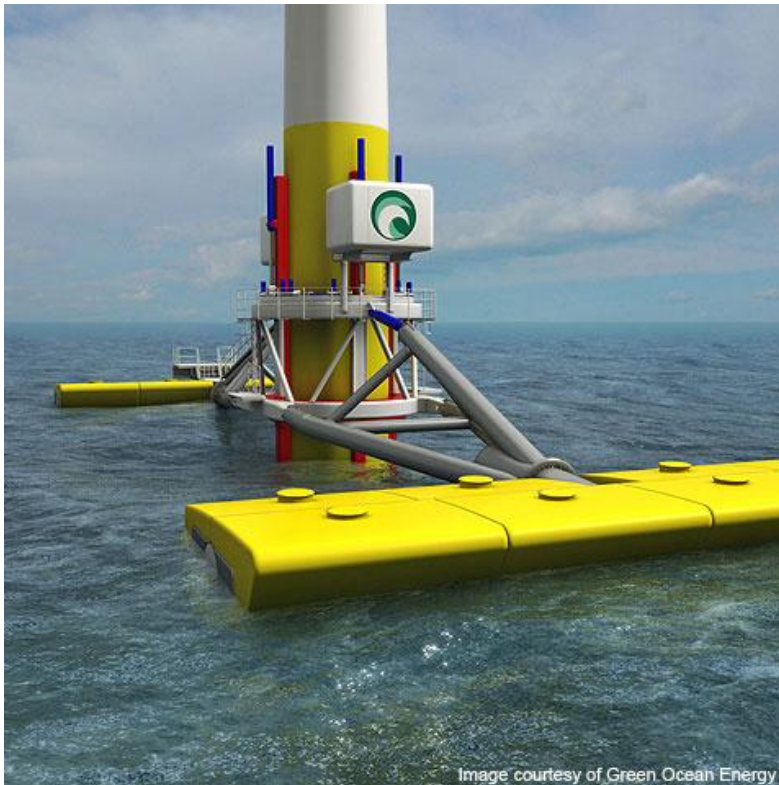
Figure 9: Conceptual design of the Wave Treader of Green Ocean Energy, attached to the monopile of an offshore windmill..
