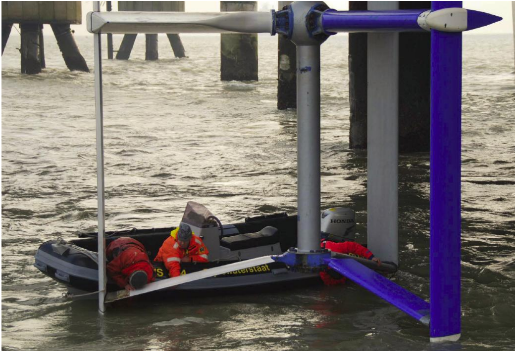
Figure 15: Inspection of the Ecofys Waverotor blades (Borsselle, the Netherlands), Picture by Peter Scheijgrond.
