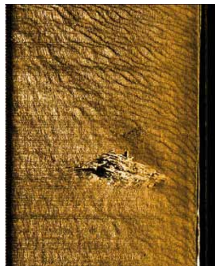
FIG. 7 Side-scan sonar van de Buiten Ratel-wraksite en de omgeving. © Afdeling Kust - Vlaamse Hydrografie. Side scan sonar image of the wreck site and surrounding area. © Afdeling Kust - Vlaamse Hydrografie.
