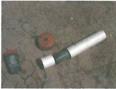
Figure 2.5 Corer used for benthic sampling. The small ones for mesocosm experiments and the larger one for field experiment (with floating system (re-designed by Yagual, G., 2004)
