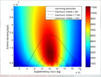
Absorbed power [W] as a function of external damping and supplementary mass with implementation of slamming and stroke limitations for  $H_{\xi}$  values between 1 and 1.5 m. The buoy is a cone-cylinder with diameter of 4m and draft of 3 m. The area enclosed by the contour lines has to be avoided in order to satisfy the restrictions.
