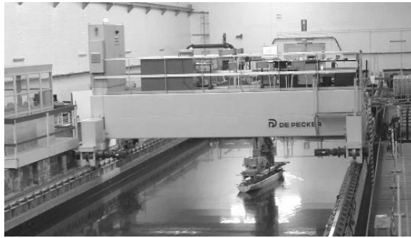
Fig 1. Flanders Hydraulics Research: towing tank for captive manoeuvring tests in shallow water.
