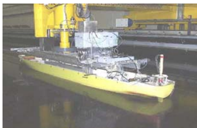
Figure 2. Ship model during captive manoeuvring test.
