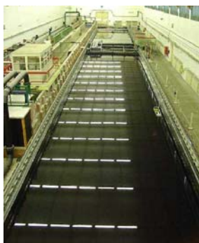
Figure 1. Towing tank for manoeuvres in shallow water.
