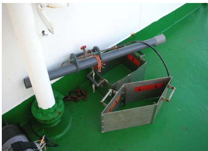
Photo 2 New foldable design frame
