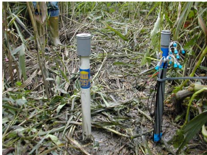
Fig. 9.3. Experimental setup at Kramp (left: perforated groundwater monitoring pipe to measure water table level, right: tube with fixed Rhizon soil moisture samplers to sample pore water at multiple sampling depths)
