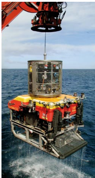
Deployment of Isis deep ocean ROV
