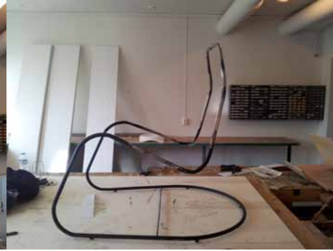
attempt n2: bending forward the headrest it was almost good a part for the fact that most of the people were clashing on the metal pipe.
