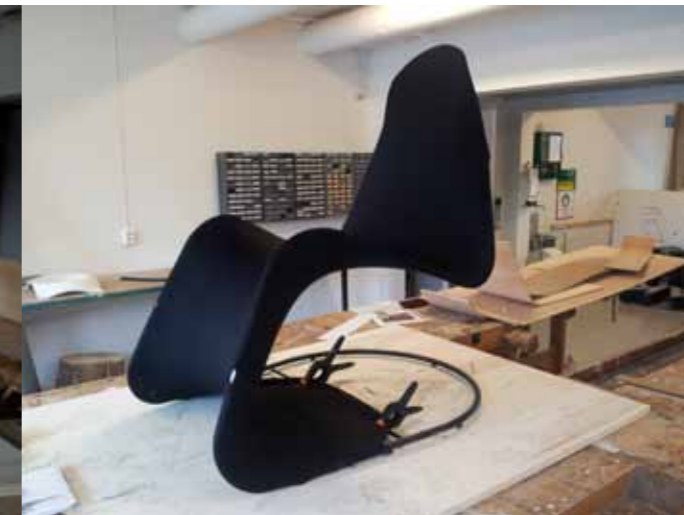
attempt n4 : A double bend seems to create a sort of notch that accommodate the head without pressing on the neck. Shoulder and back are comfortable too but bending the pipe back the height of the headrest decreased.
