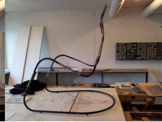
attempt n5 : By increasing the height of the headrest the chair seems to fit most of the body types delivering a very comfortable position.
