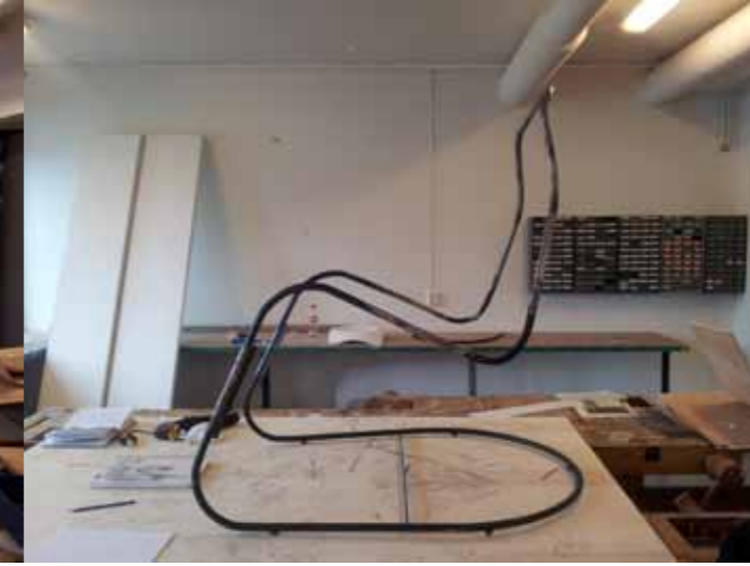
attempt n4 : A double bend seems to create a sort of notch that accommodate the head without pressing on the neck. Shoulder and back are comfortable too but bending the pipe back the height of the headrest decreased.
