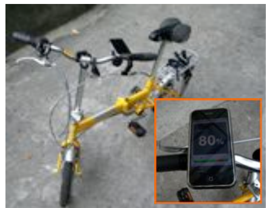
Figure 2. The mobile is placed at bike stem; it senses acceleration data when bicycling, and infers terrain and stamina cost.
