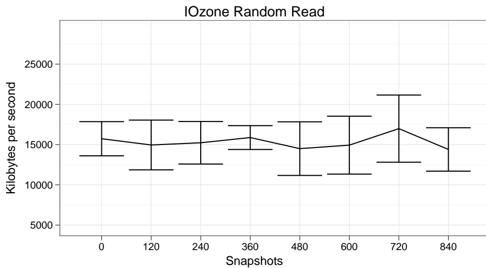
Figure 6.22: Plot of Hammer: IOzone 'random read'. The x-axis is number of snapshots; the y-axis is KB/s.
