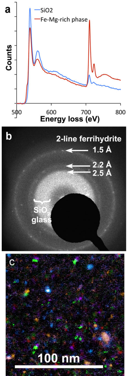
Fig. 5. a) EELS spectra from a relatively large silica nanoparticle (blue) and from its shell (red), concentrating on the region around the O-K edge at \sim 532 eV and the Fe-L 2,3 edge around 708 eV. b) SAED pattern from a group of nanoparticles showing features consistent with a mixture of two-line ferrihydrite and amorphous silica (labeled SiO 2 glass). c) A composite of several dark-field TEM images of Fe-Mg silicate produced using the 2.2 Å diffraction ring, which shows that the ring has been formed by scattering from many ferrihydrite nanocrystals.
