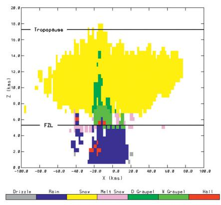
FIG. 10. Cross section of C-Pol data near Darwin (17.5 km south of Gunn Point) at 1550 UTC 12 Jan 2003 showing the precipitation classification. Dry and wet graupel are shown separately as D and W Graupel. The freezing level is at 5.3 km, and the tropopause at 17.3 km.
