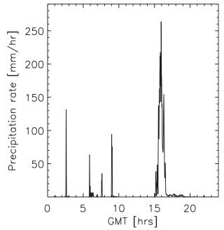
FIG. 3. One-minute rainfall measurements from the ARM rain gauge in Darwin on 12 Jan 2003.
