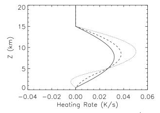
FIG. 11. Local profile of latent heating in a 100 mm h<sup>-1</sup> deep convective rain event. The solid line shows the heating profile assuming only moist rain with no evaporation. The dashed line shows the profile assuming ice above the melting layer, and the dotted line shows the effect of assuming that 30% of the rain in the column evaporates below 5 km.
