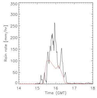
FIG. 5. The Darwin ARM-TWP 1-min rain gauge measurement for 12 Jan 2003 (black) and the C-Pol radar 10-min rain rate for the grid point closest to the rain gauge location (red).
