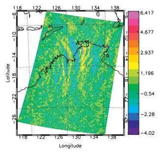
FIG. 1. AIRS radiance perturbations, defined as the difference from a fourth-order polynomial fit in scan angle that removes the scan angle dependent radiance. This is a granule from channel 75, in the 15- $\mu$ m region, centered on wavenumber 667.78 cm<sup>-1</sup>. The data were acquired over northern Australia at 1640 UTC 12 Jan 2003 and the radiance units are mW m<sup>-2</sup> sr<sup>-1</sup> cm.
