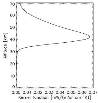
FIG. 2. The temperature kernel function for AIRS channel 75.
