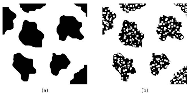
Fig. 5 The role of percolation at the contact interface (schematic). (a) Area of contact as it appears when the contact is observed at the magnification \zeta . (b) The real area of contact (observed at the highest magnification \zeta_1 ) corresponding to Fig. 5(a).
