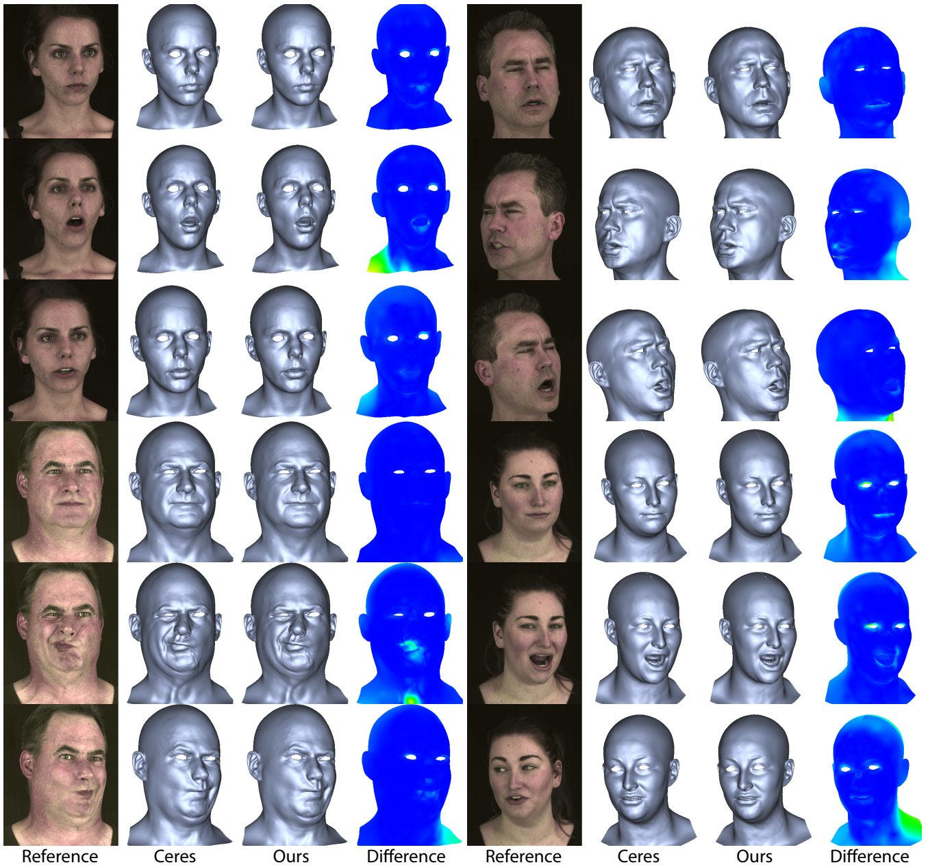
Figure 12: We demonstrate the accuracy of our fast nonlinear solver with the application of facial capture using an anatomical local model (ALM), and compare to the same result solved using the Ceres solver [AMO]. Here we show 3 frames from sequences of 4 different actors. The reconstruction results differ only very little, as illustrated in the heatmap (from blue=0mm to red=0.2mm), and the majority of the difference is in the back of the head and shoulders where there is no data to constrain the optimization. Despite nearly identical results, our method ran 10 times faster per face solve, and each frame contained 8 iteration of solving, yielding a significant speedup.
