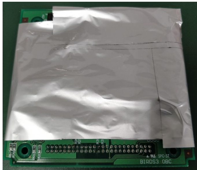
Figure 66. BIRDS-4 OBC board wrapped with commercially available EMI shielding/absorber sheet
