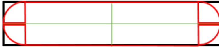
Figure 4.30 – Mathematical modelling of the rod shape of E. coli cells (red colour). Minor and Major Axis in Green. The semi circles have a radius defined as half of the minor axis.
