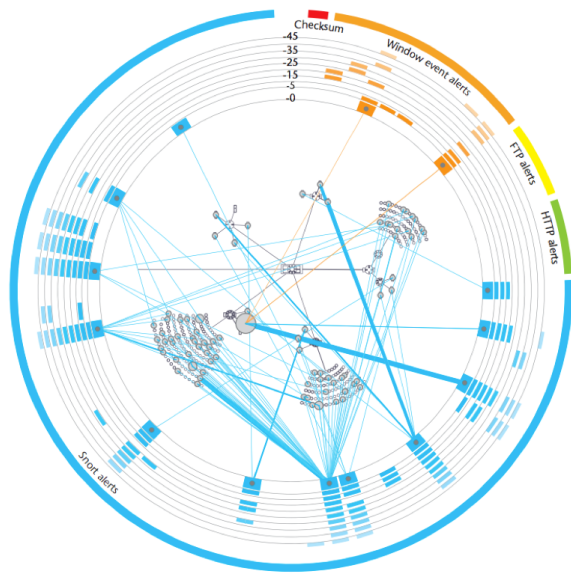
Figure 10. VisAlert visualization [102]. In the center of the circle is a graph layout of the network. The circle's radial sections moving from most recent (closest to the topology map) to the least recent determine the alert type.
