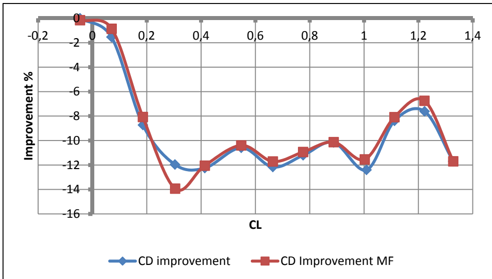
Figure 5.13 Drag coefficient reduction over the lift coefficient range for Mach = 0.20
