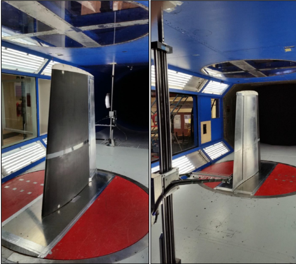
Figure 8.9 MDO 505 wing model setup in the wind tunnel test section
