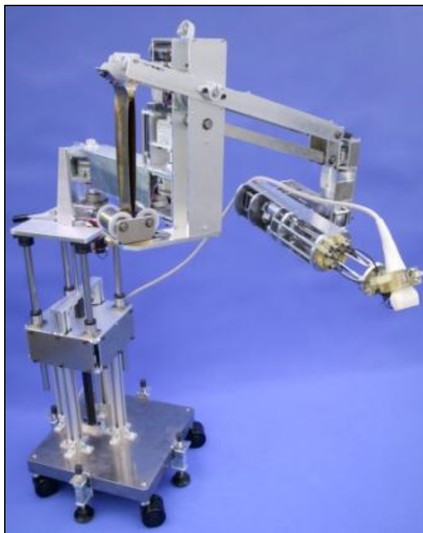
Figure 1.6 WTA-2R, a robot system for carotid ultrasound diagnosis (Nakadate et al., 2009)
