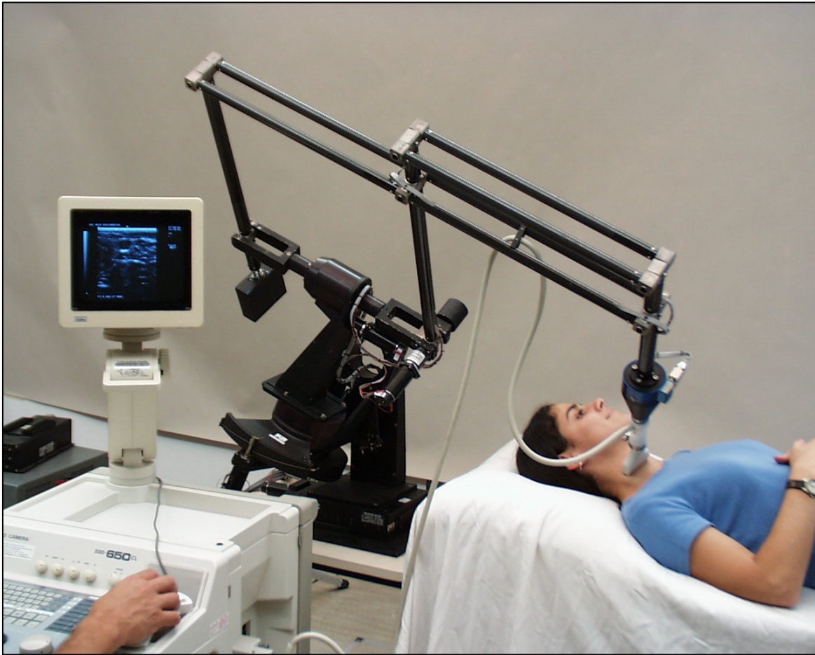
Figure 1.8 A fully-balanced medical US robot from University of British Columbia (Abolmasesumi et al., 2002)
