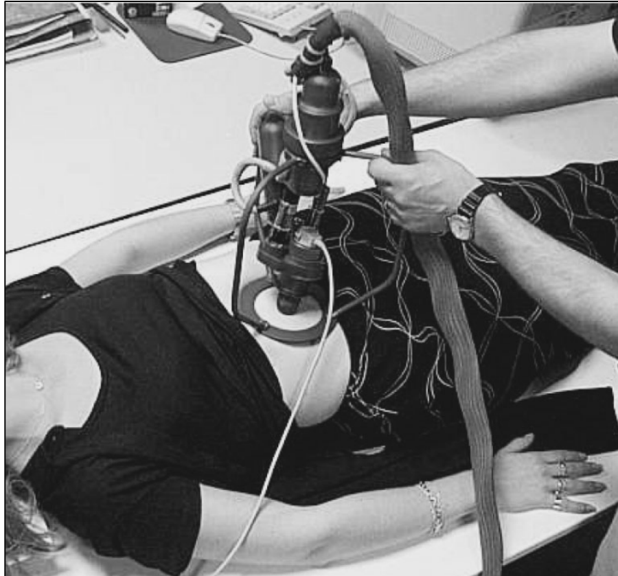
Figure 1.3 The TERESA robot in US scanning, held by a paramedic (Vieyres et al., 2003)
